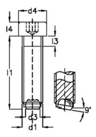
$\begin{array}{lll} d1 & = M6 \\ d2 & = 4.0 \\ d3 & = 3.2 \\ d4 & = 10 \\ Internal \ hexagon = 5.0 \\ I1 & = 30 \\ I3 & = 3.0 \\ I4 & = 6 \end{array}$
